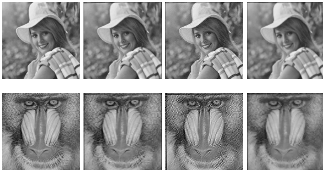
(a) (b) (c) (d) Figure 1 : Simulation Results: column (a) HR Test Images, (b) Results using Bicubic Interpolation, (c) Results using IBP, (d) Results using POCS Method
