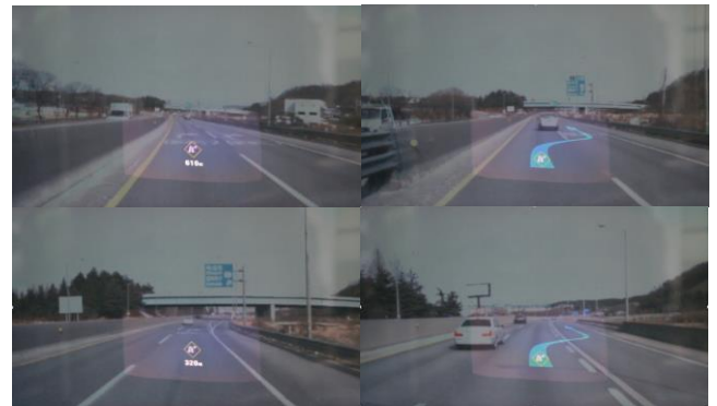
Figure 5. Lane Change Guidance on the Highway
