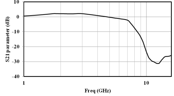
Fig. 6. Normalized S21 measurement result of the proposed TIORx module.
