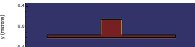
Fig. 17. Mode profile at core width of 500nm and core height of 300nm.
