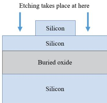
Fig. 2. The geometry of rib-type based waveguide on SOI platform.
