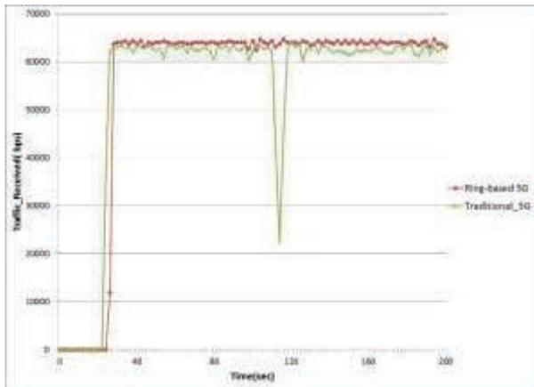
Fig. 8. Traffic Throughput during UE handoff
