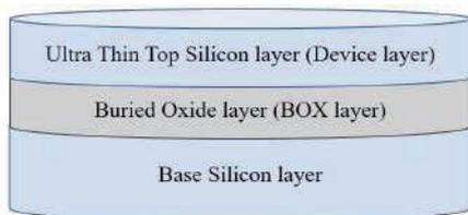
Fig. 1. SOI wafers.
