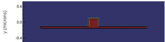
Fig. 4. Mode profile at core height of 200nm and core width of 300nm.
