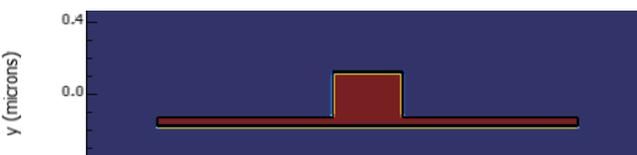
Fig. 16. Mode profile at core width of 500nm and core height of 250nm.
