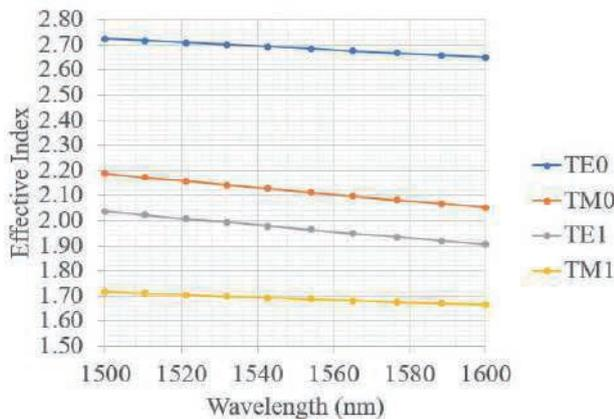
Fig. 11. Graphs of Effective index at height of 200nm with width of 600nm for 4 modes.
