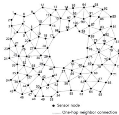
Fig.5. Constructing a sensor network with Voronoi polygons
