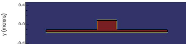
Fig. 15. Mode profile at core width of 500nm and core height of 200nm.
