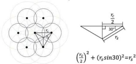
Fig. 4. Model of sensing radius and transmission radius
