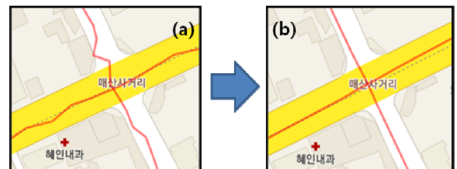
Figure 9. Final road map data created by exterior adjustment of formed road link data: (a) before adjustment: (b) after adjustment
