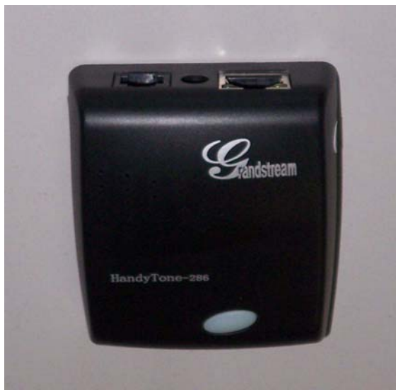
Figure 4 Grandstream HT286 as VoIP Adaptor
