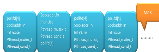
Figure 8. Data structure for the multicast area
