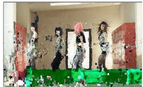
(c) Video frame sample with packet loss due to insufficient bandwidth
