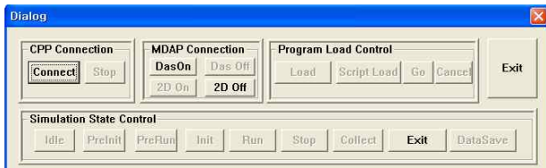
Figure 7. GUI for HWIL simulation state control
