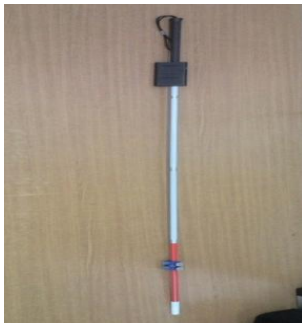
Fig. 5. The white stick using ultrasonic sensor.
