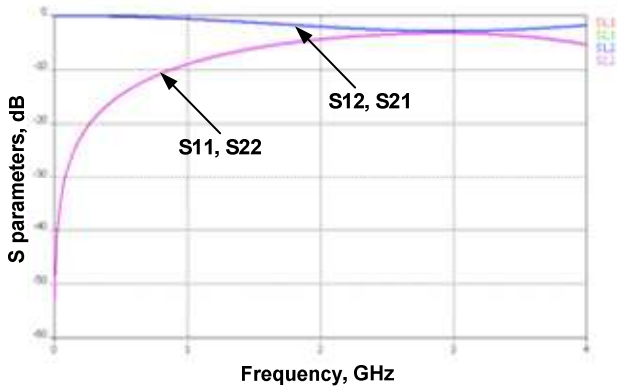
Figure 10. S-parameters of the semi-stacked spiral inductor structure
