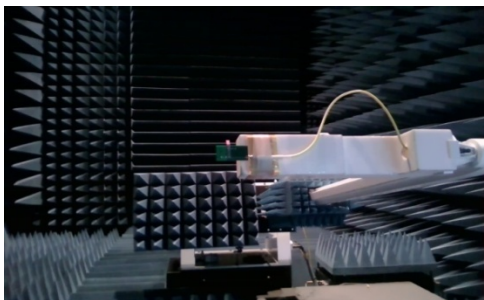
Figure 4. Measured 2.45GHz Chip ANT in anechoic chamber
