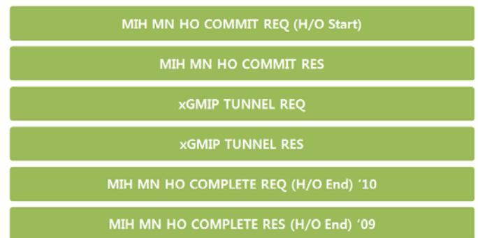
Figure 3. The procedure of IP handover between heterogeneous networks
