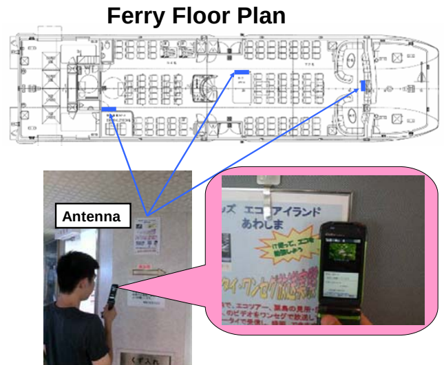
Figure 8. Installation Location within the Ferry.
