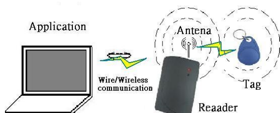
Figure 1. The concept of RFID operation.
