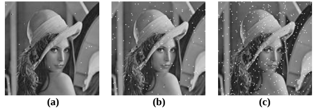
Figure 5. Reconstructed images with rate=0.5bpp and SNR=1.5dB (a) UEP (b) EEP1 (c) EEP2
