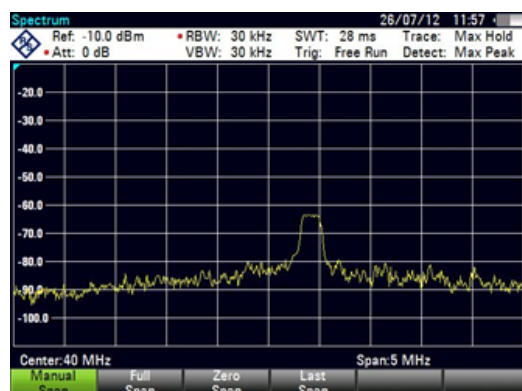
Figure 12. Adjacent Radar Waveform
