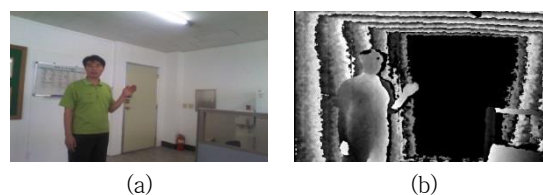
Figure 4. The process of Separating the Foreground from the Depth Image
