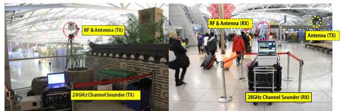
(b) Installation of measurement equipments
