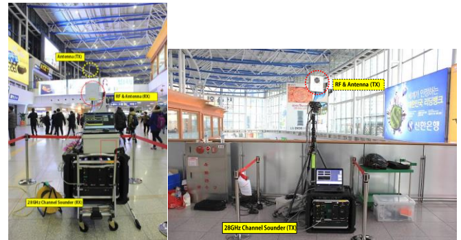
(b) Installation of measurement equipments
