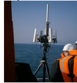
Figure 9. Prototype of Directional Antenna Tracking Module
