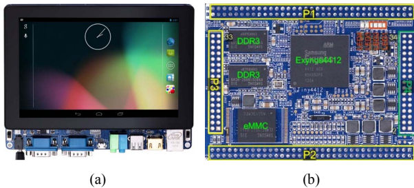
Figure 9. Tiny4412 platform (a) Outlook of the Tiny4412 platform; (b) The core board of Tiny4412 platform
