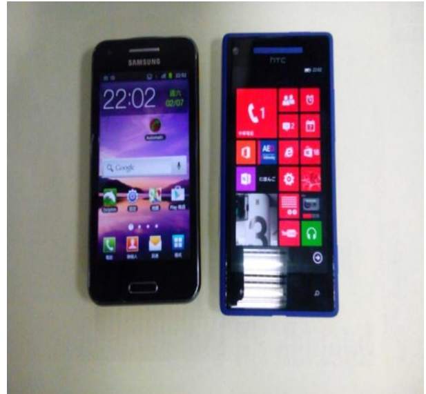
Fig. 1. The smart phones: Galaxy Beam, GT-I8530, Samsung™ as transmitter, and Windows Phone 8X, hTC™ as receiver.
