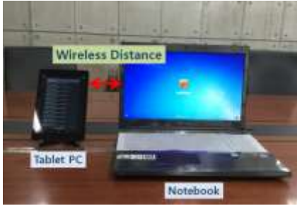
Figure 1. The relationship test between near field distance and Bluetooth RSSI in a meeting room environment.
