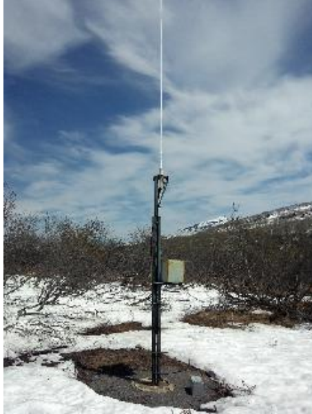
Figure 2. Some types of antennas used in IKIR [8] for whistler detection and lightning localization
