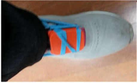
Figure 5: IMU attached the to user's right shoe
