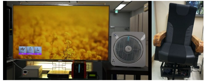
Figure 4. Sensory effect representation devices synchronized with AV
