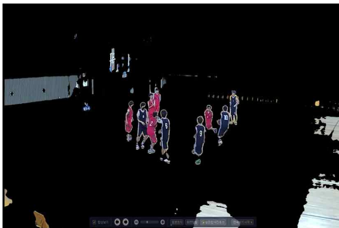
FIGURE 2: BACKGROUND SUBTRACTION The foreground region is extracted by subtracting an input image by the background image
