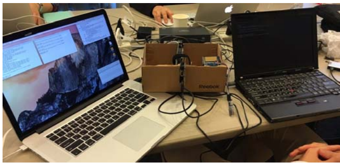
Figure 5. Testbed for IPv6 networking between two NFC-enabled devices
