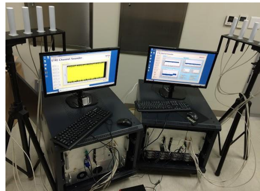
Figure 1. Developed Channel Sounder System Shape
