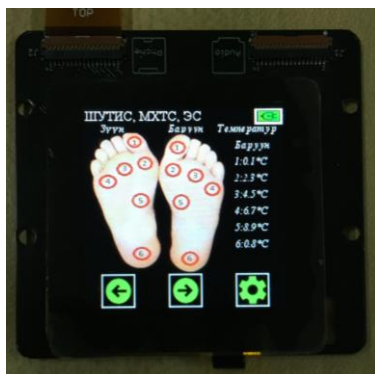
Figure. 9. User interface of healthy wearable device for monitoring of foot temperature
