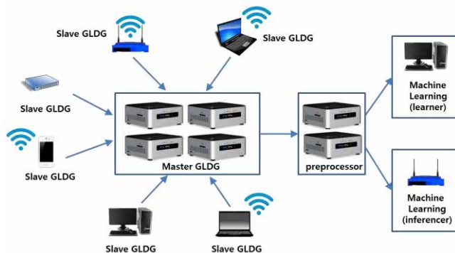
Figure 3. The system configuration of the GLDG framework
