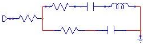
Figure 2. MBVD Equivalent Circuit
