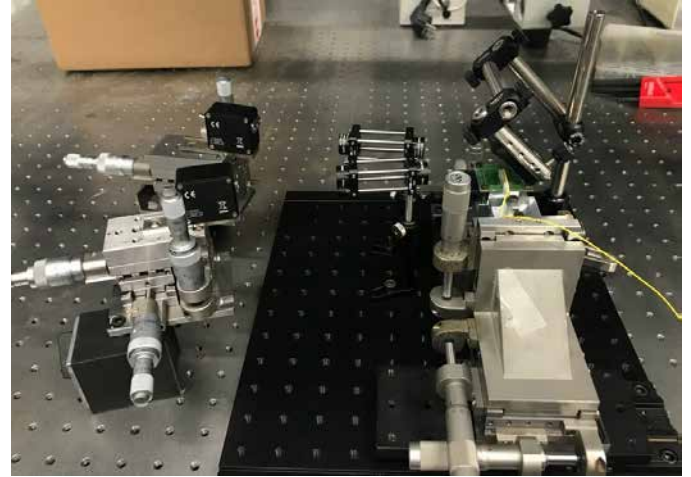
Figure 6. Experimental setup used to demonstrate high speed data transmission using packaged OPA.
