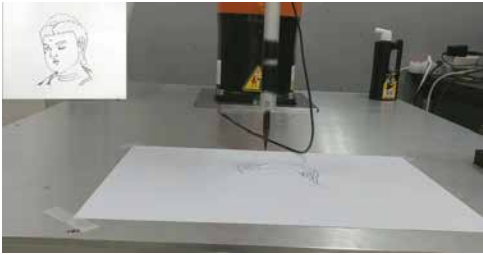
Fig. 6: Drawing imitation by a robot.
