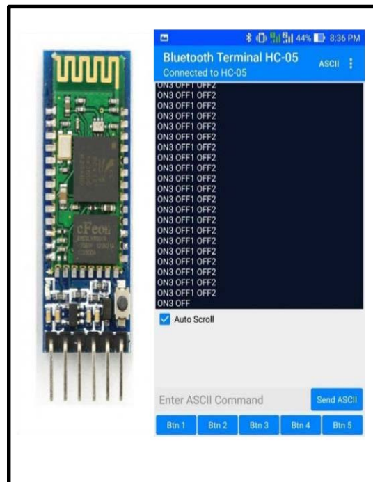
Fig. 4. An HC-05 module used with Arduino(on the left) & sensor status data received from Arduino on the CDRM over Bluetooth channels
