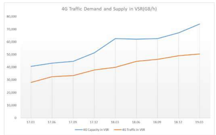
Figure 5. 4G traffic volume and system capacity in VSR
