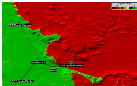
Figure 3. Base Station (BS) radio coverage single polar
