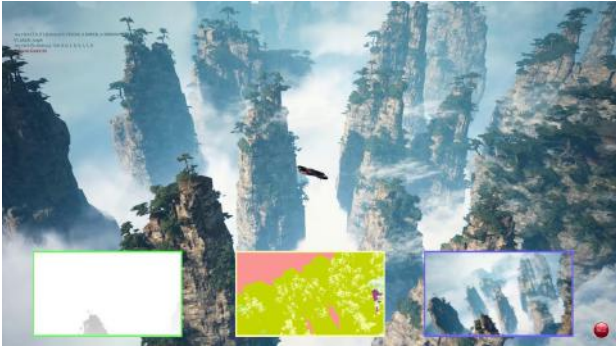
Fig. 1. Image from an AirSim simulation including a UAV model, front-facing of the UAV and sensors.
