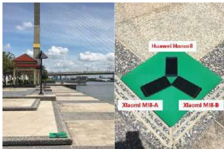
Figure 7. Setup of Smartphone on top of a ESD rubber sheet at Reference coordinate (The Rama VIII bridge park in Thailand).
