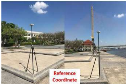
Figure 6. Setup of ComNav T300 Pro-GNSS receivers at Reference Coordinate (The Rama VIII bridge park in Thailand).
