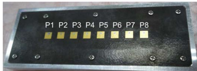
Figure 1. The uniform linear antenna array with evenly spaced patch antenna elements (P1 – P8) aligned in the horizontal direction.
