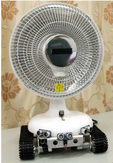
Figure 3. The user's temperature tracing voice-controlled movable electrical heating radiator.
