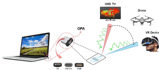
Figure 1. Architecture of optical wireless data transmission through an optical beam steering module based on optical phased array and applications.
