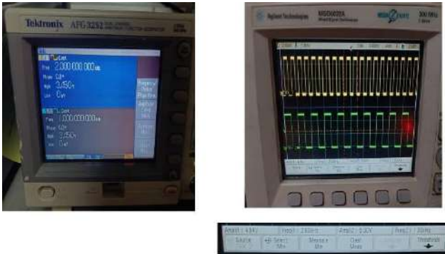
Figure 11. AWG Generated Waveform (L), MSO Captured Waveform (R)
