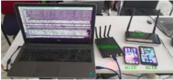
Fig. 4: Test and validation system
