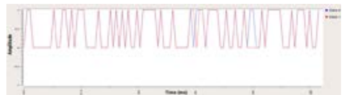
Figure 22. Comparison between demodulated signal and original signal
