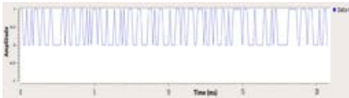
Figure 19. Symbol after 1-bit differential demodulation decision
